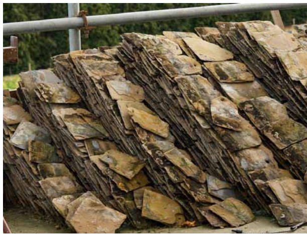
Collyweston Slate used extensively in Stamford, Lincolnshire (© English Heritage/J Humble)
